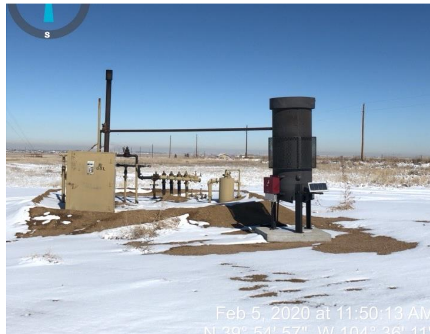
Photo #2 separator and combustor
