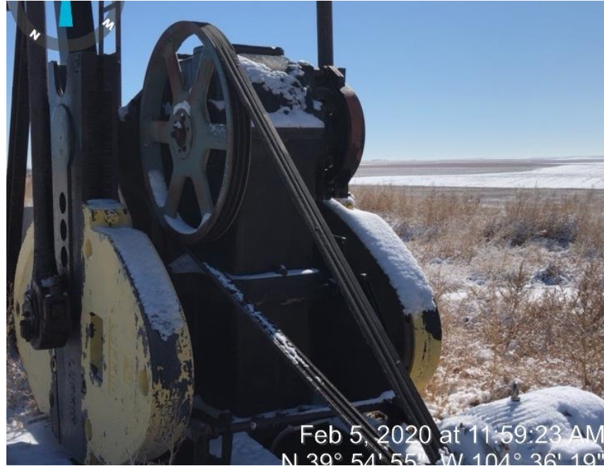
Photo #13 safety equipment not in place on pumpjack
