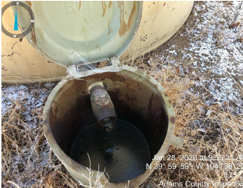
Photo #3 bull plug missing from load out line
