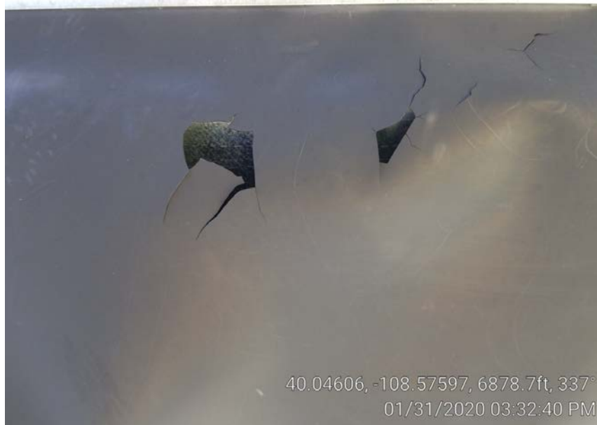
Photo 4. Tank line hole on 1-31-2020.
