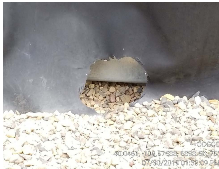
Photo 5. Tank liner hole on 7-30-2019.
