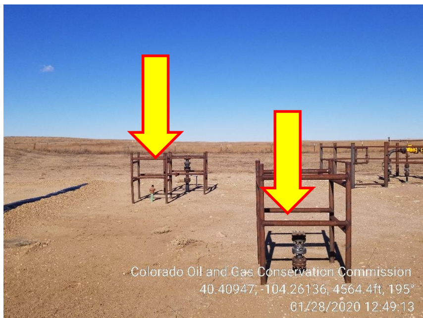
Photo 6 – Unmarked Risers and the North side of Location
