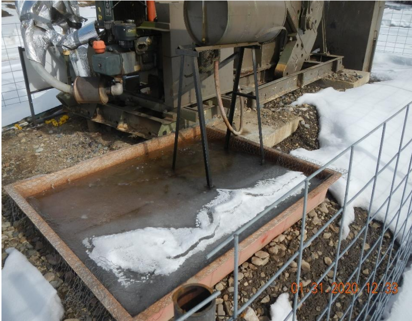
Inadequate secondary containment for lube oil container.
