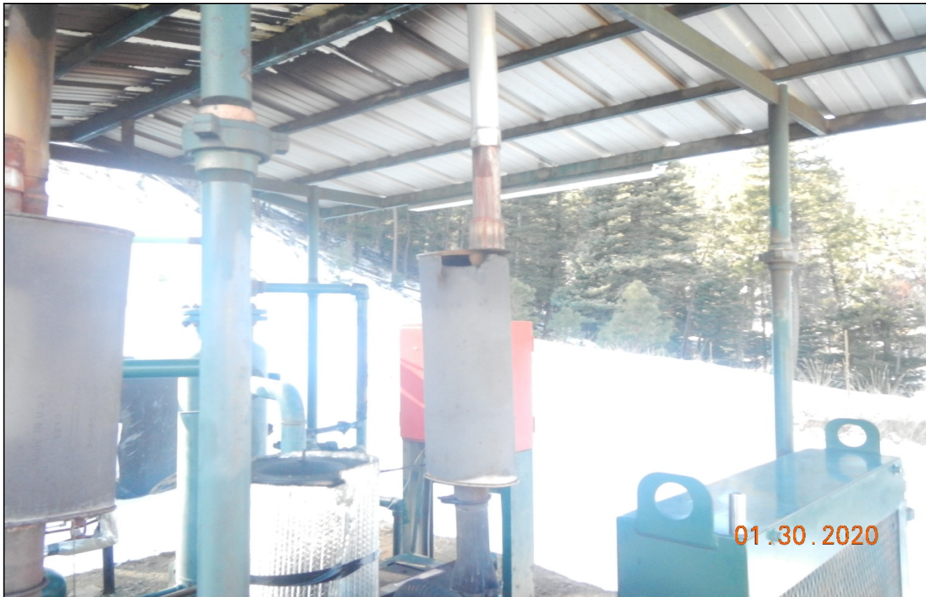
Photo 5. The muffler on the engine is broke apart causing the engine to be very loud. Needs to be maintained in good mechanical condition.
