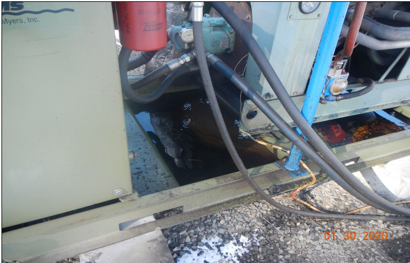
Photo 3. There is oily waste in the engine skid.
