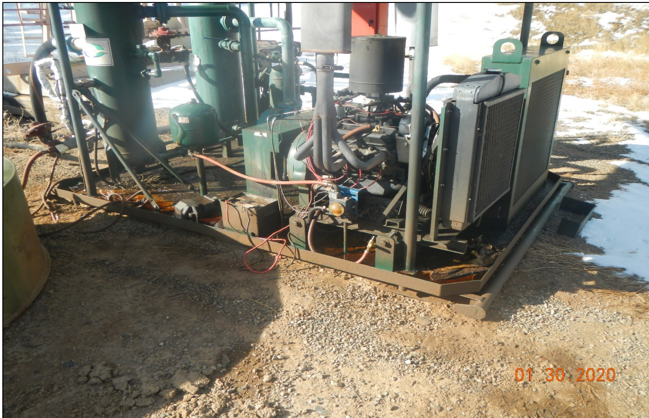
Photo 6. There is oily waste at the engine skid at the separator.
