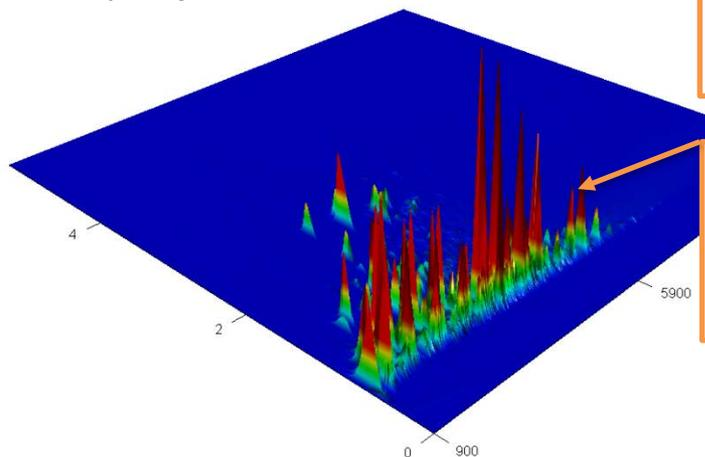
**Important:** Compounds present in soil extracts very similar for all samples except SB03 (not shown here). Differences in relative peak heights reflect concentration of hydrocarbon contaminant in soil.
