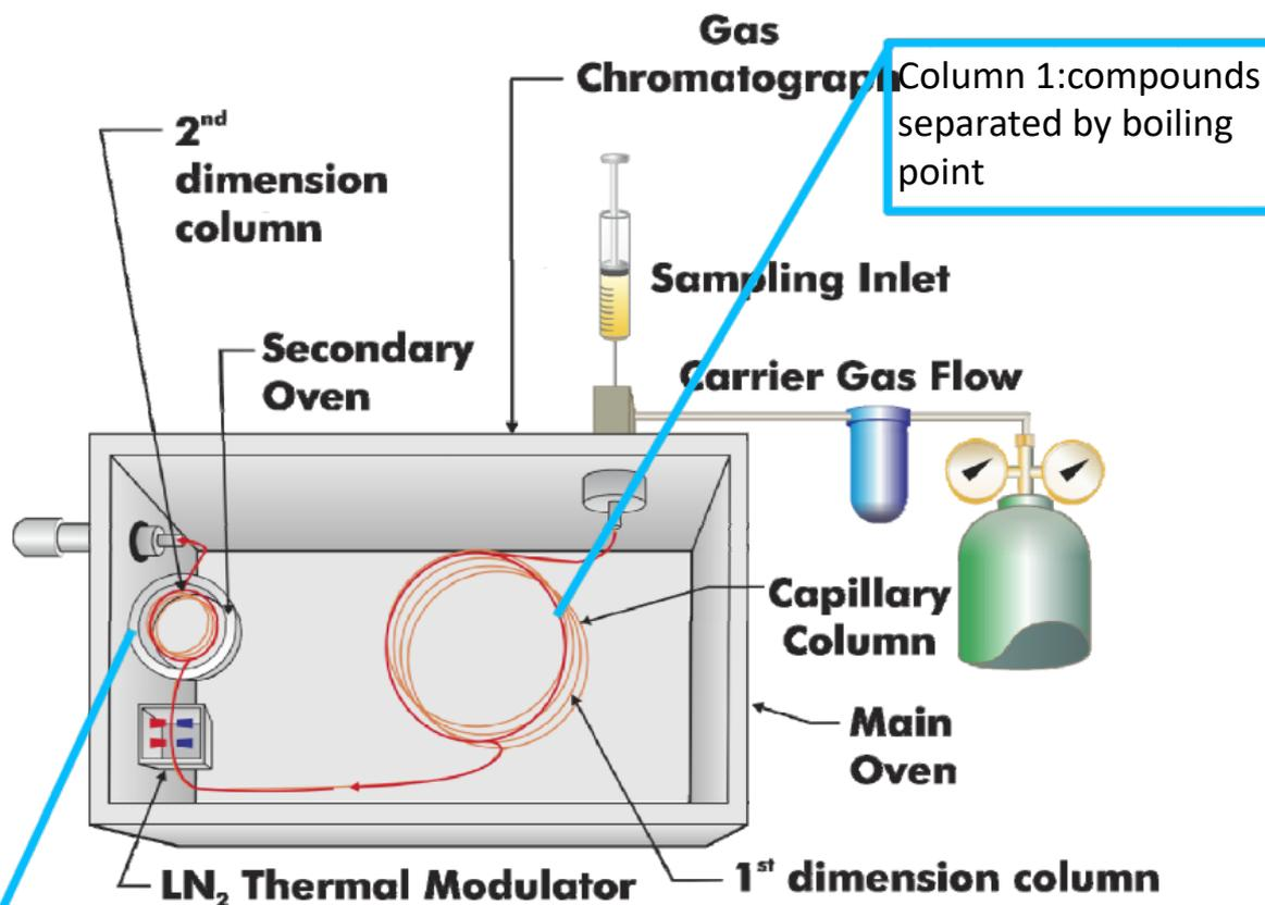
Can be equipped with a Flame Ionization Detector (FID) or Time of Flight Mass Spectrometer (TOFMS) for more comprehensive molecule identification
