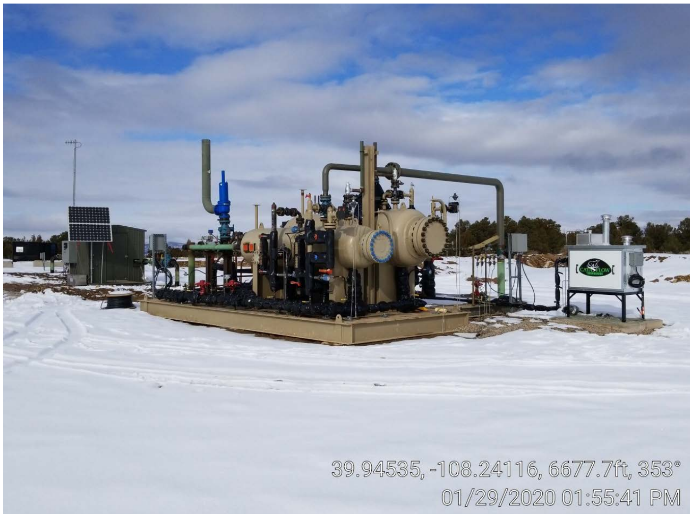
Photo 3. Separator & meter building.
