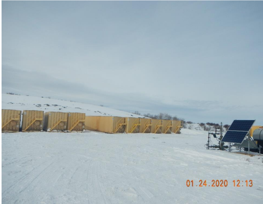
Approximately 60 500 bbl frac tanks on location.
