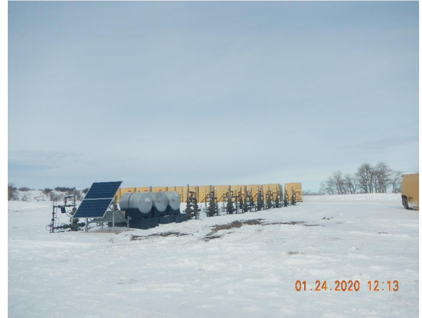
Approximately 60 500 bbl frac tanks on location.
