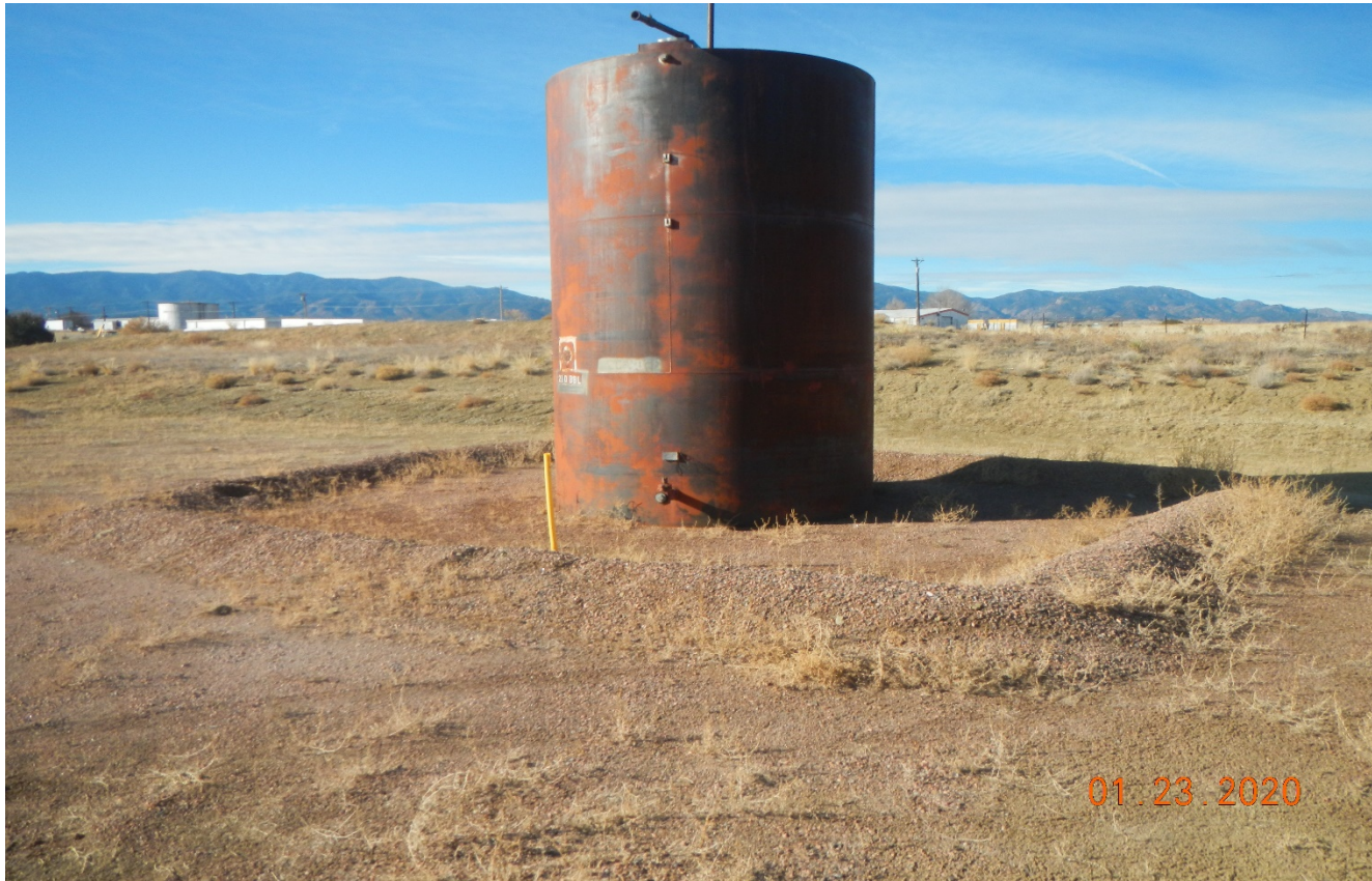
Photo 7. The tank does not have the required labeling.
