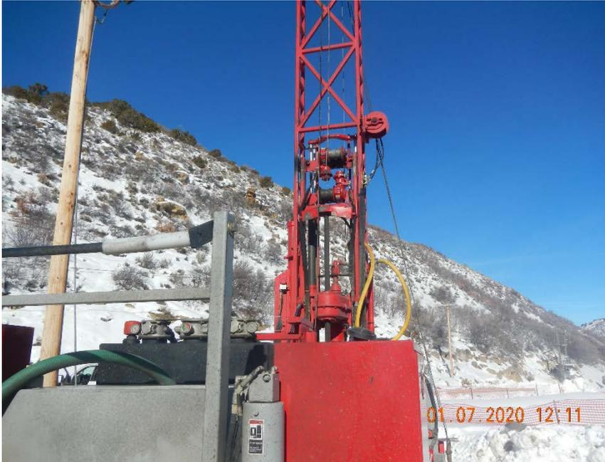
Photo #9 Rig that was used for groundwater investigation.
