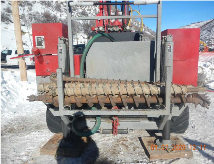
Photo #8 Rig that was used for groundwater investigation.
