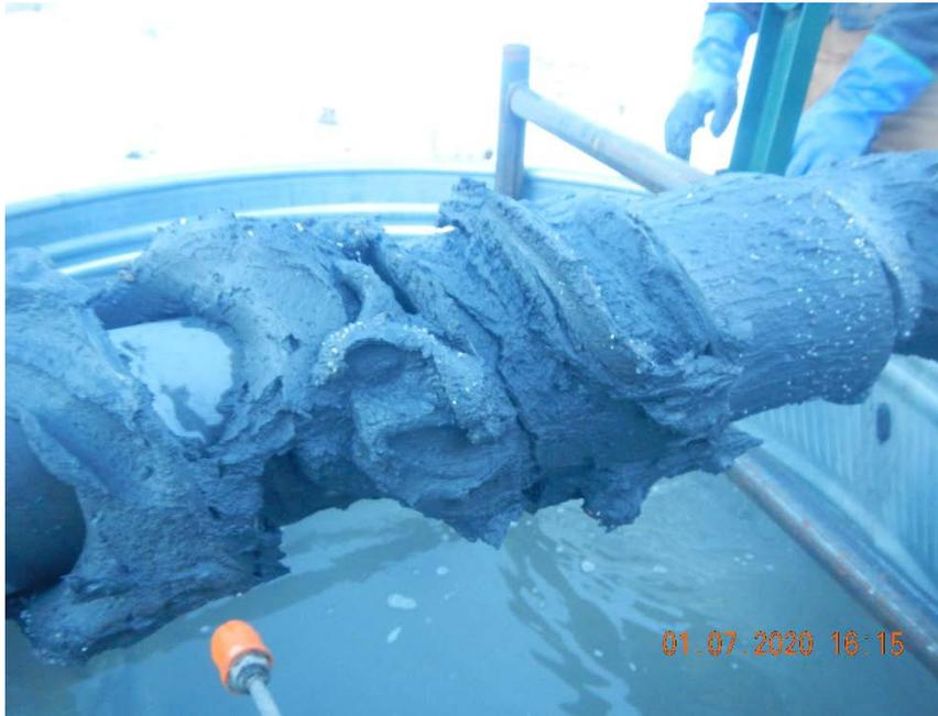
Photo #24 Cleaning of auger bit. Note: kiddie pool catchment basin.
