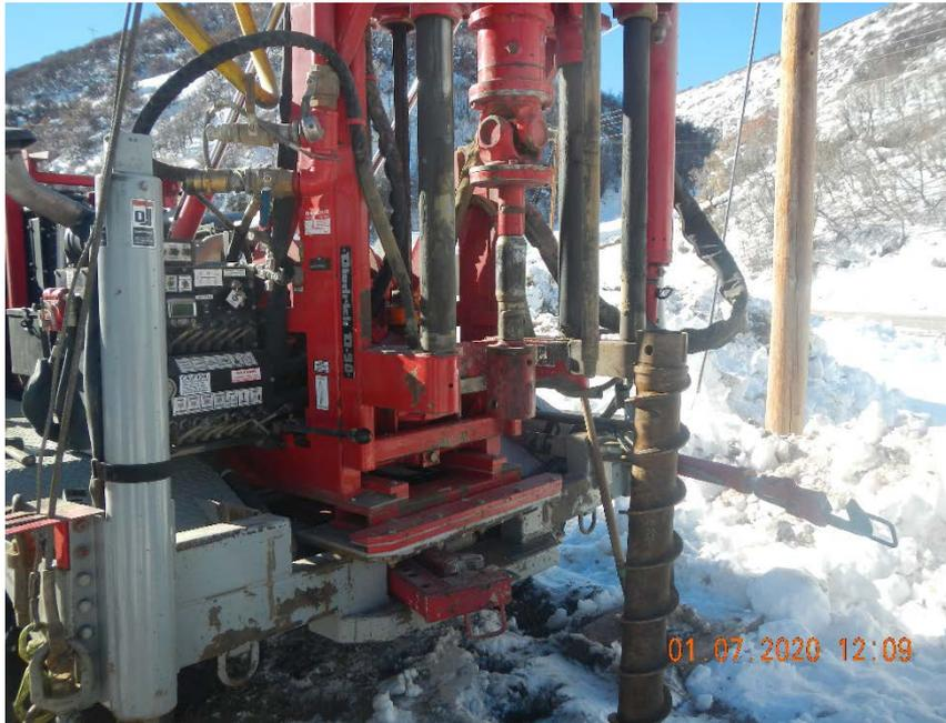
Photo #5 wellhead Rig that was used for groundwater investigation. Diedrich D-90. Rig was owned and operated by HRL Compliance Solutions Inc.
