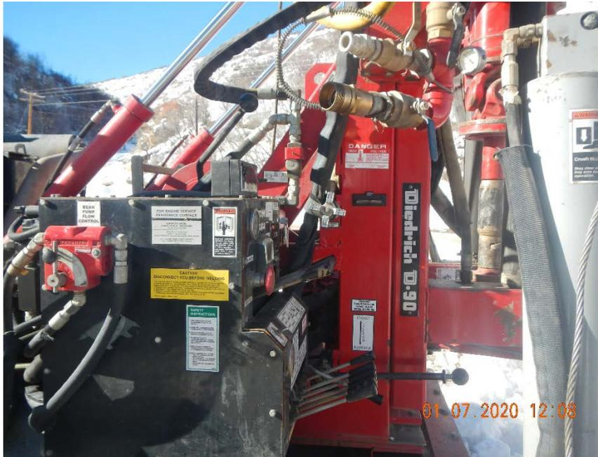
Photo #3 Rig that was used for groundwater investigation.
