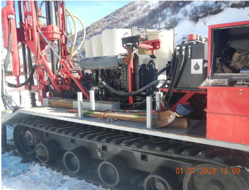
Photo #6 wellhead Rig that was used for groundwater investigation. Diedrich D-90. Rig was owned and operated by HRL Compliance Solutions Inc.
