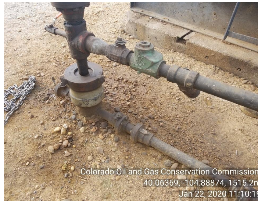
Photo 2 Stained soil around well head CO C #1
