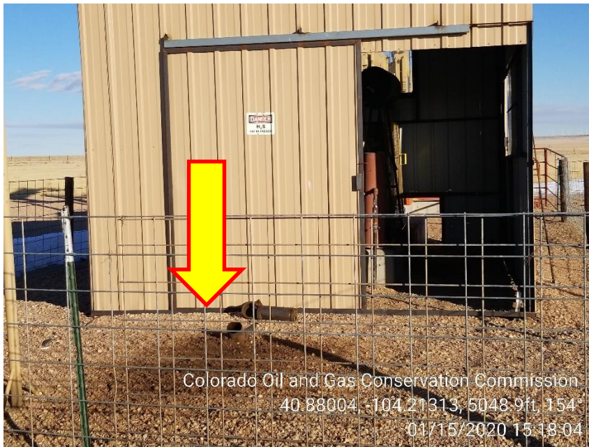
Photo 3 – Stained Soil at Exhaust
