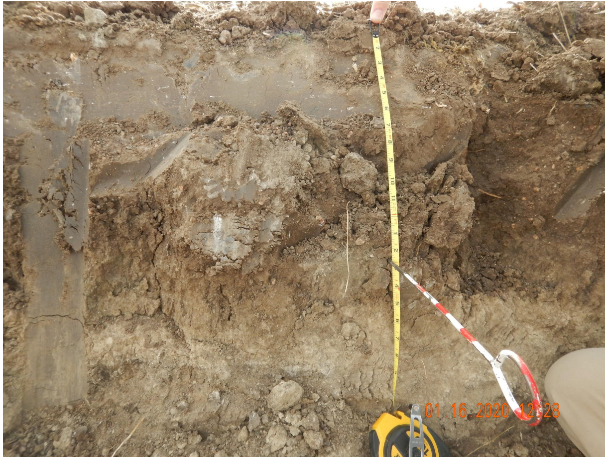
Photo 10. Photo taken from within the sediment trap located along southwestern perimeter of location. Based on field observations and physical characteristics (color, texture, structure, and primary root depth), topsoil is approximately 14 inches. Note: COGCC staff gave a conservative estimate on topsoil depth as it was observed up to 17-18
