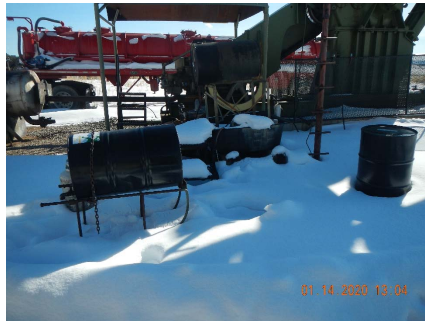
Photo 4. No secondary containment.
