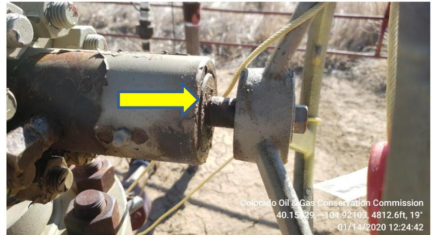
**Photo 3 Stained soil around bradenhead**
