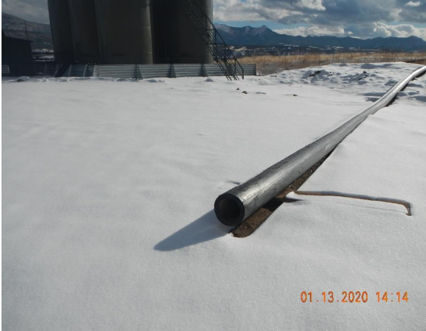
1 poly pipe water line by frac lines. Line is not capped.
