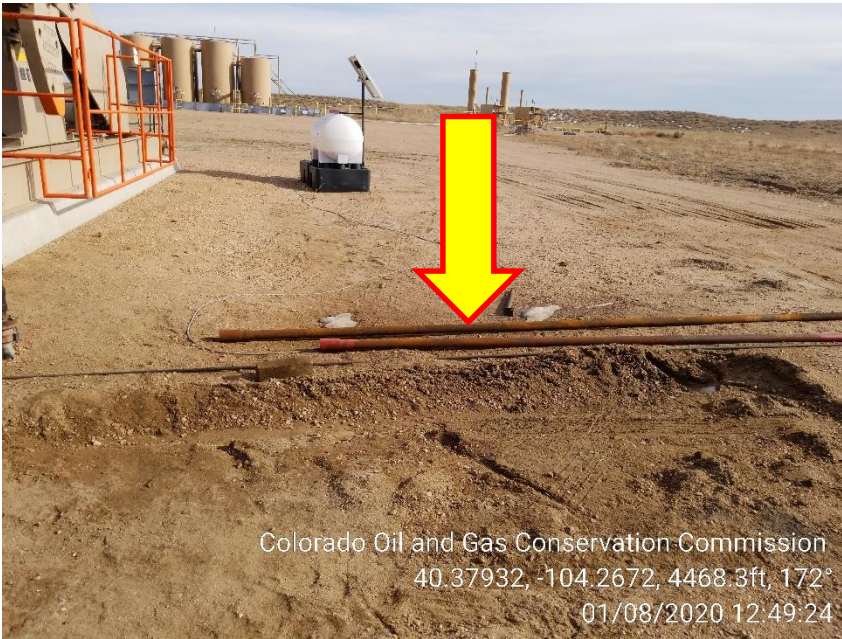
Photo 3 – Unused Tubing and Rod Strings
