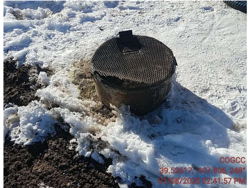
Stained soil around buckets outside of containment
