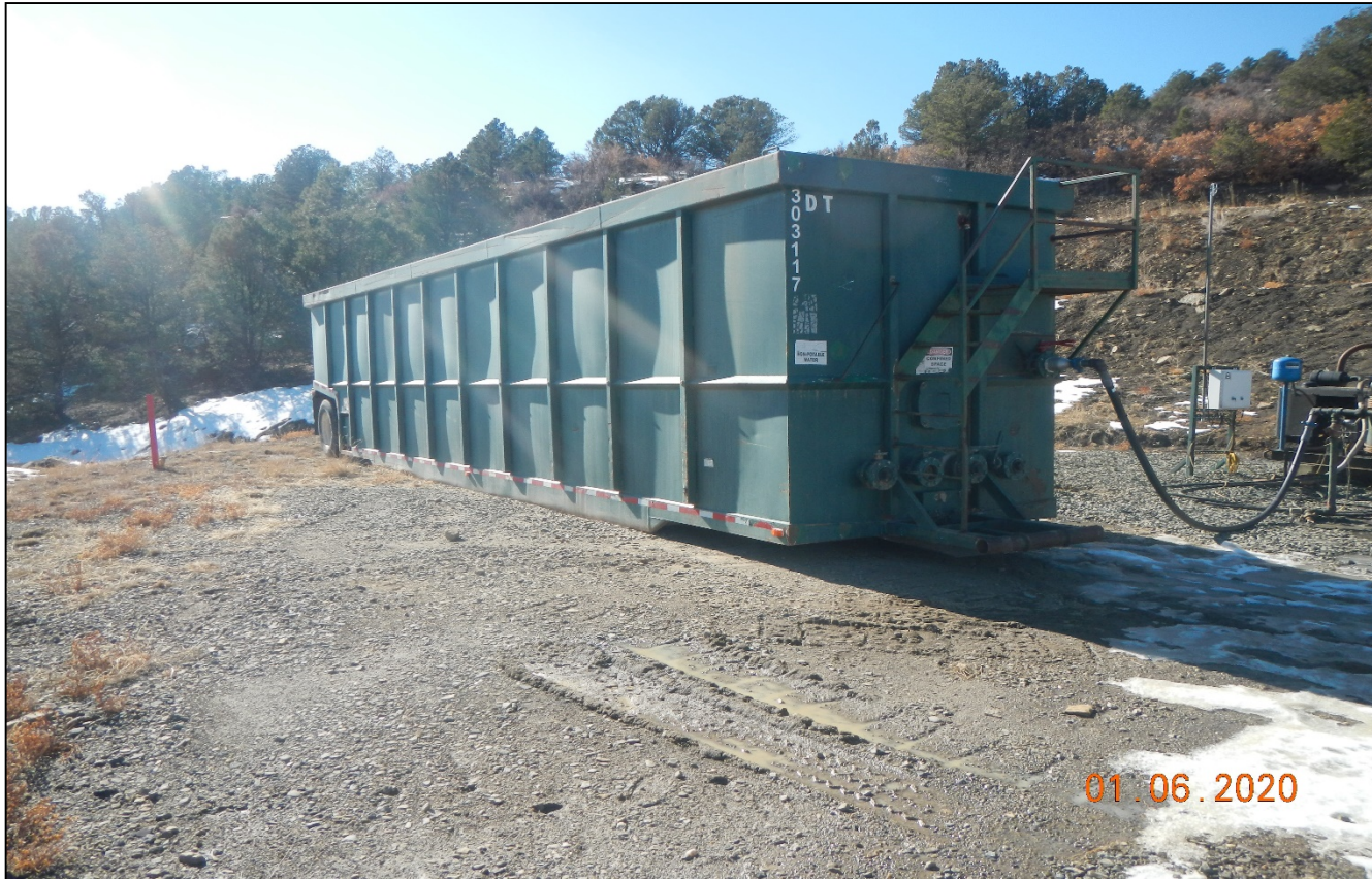
Photo 5. The tank at the location does not have secondary containment or proper labeling.
