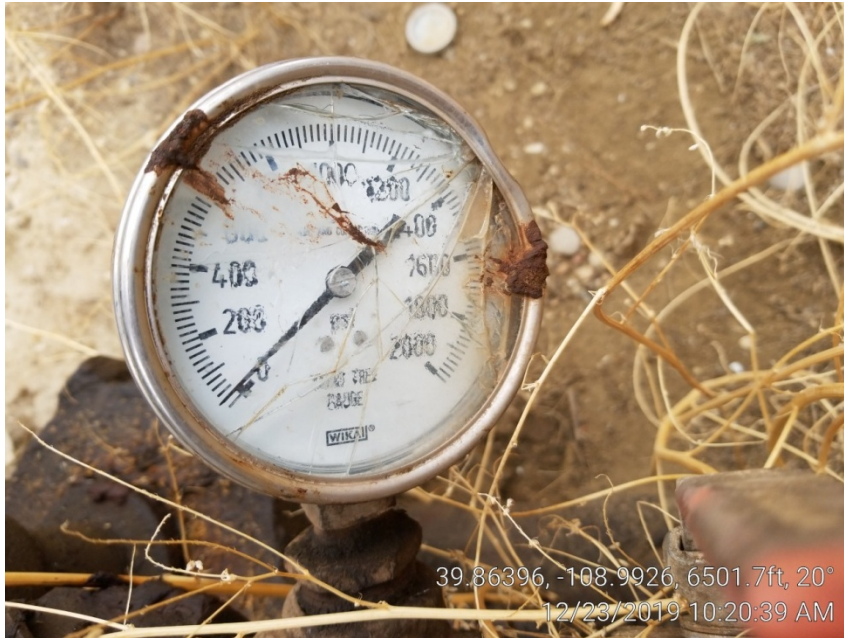
Photo 15. Casing gage @ 20 psi.
