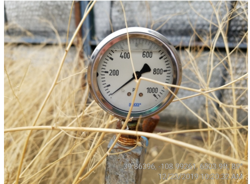
Photo 16. Tubing gage @ 40 psi.
