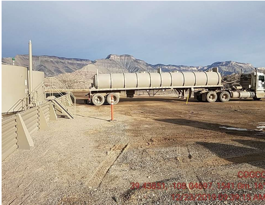
Truck on location pulling production water and no sign of a strong Oder.
