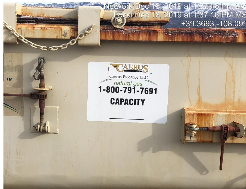
Photo #0283 Roll top tank missing capacity and contents labels.
