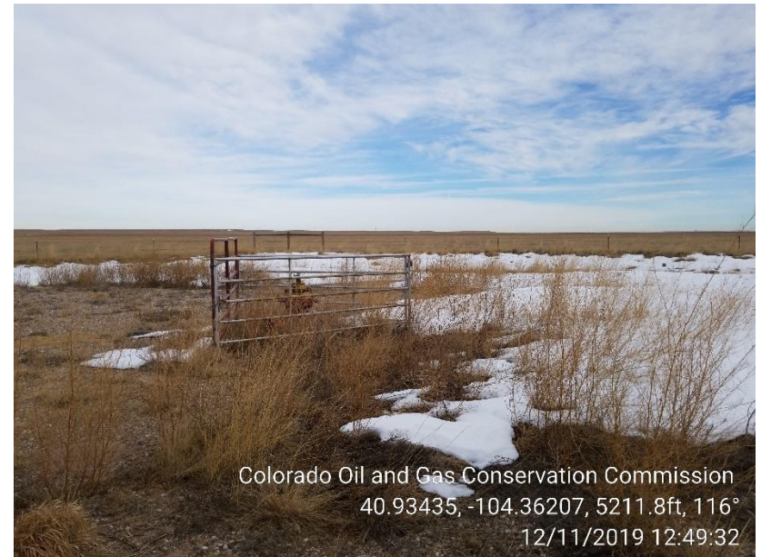
Photo 2 – Weeds at Wellhead. No Wellhead sign or Emergency contact info posted.
