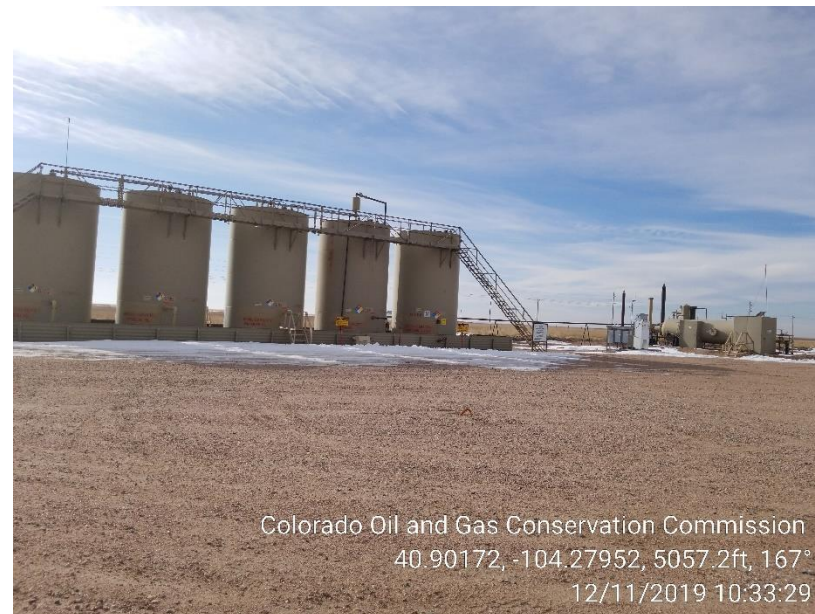
Photo 2 – Tank Battery
