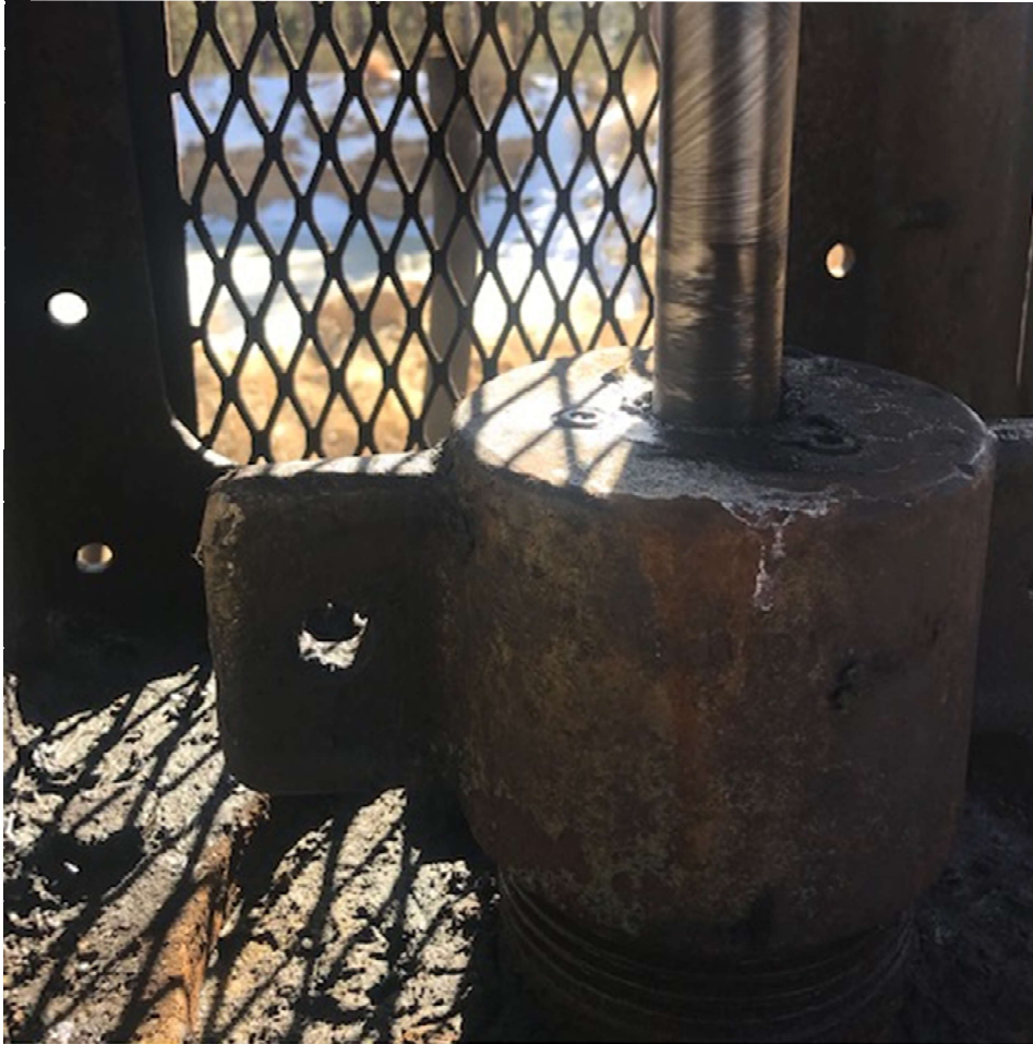
PHOTO 1: THE PACKINGS WERE CHANGED AND GREASED TO PREVENT THE WATER FROM LEAKING. THE WING NUT WAS SECURLY FASTENED TO ENSURE GOOD MECHANICAL CONDITION.
