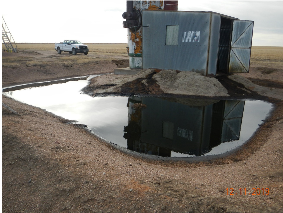
Photo # 5 – Oil spill within treater berm
