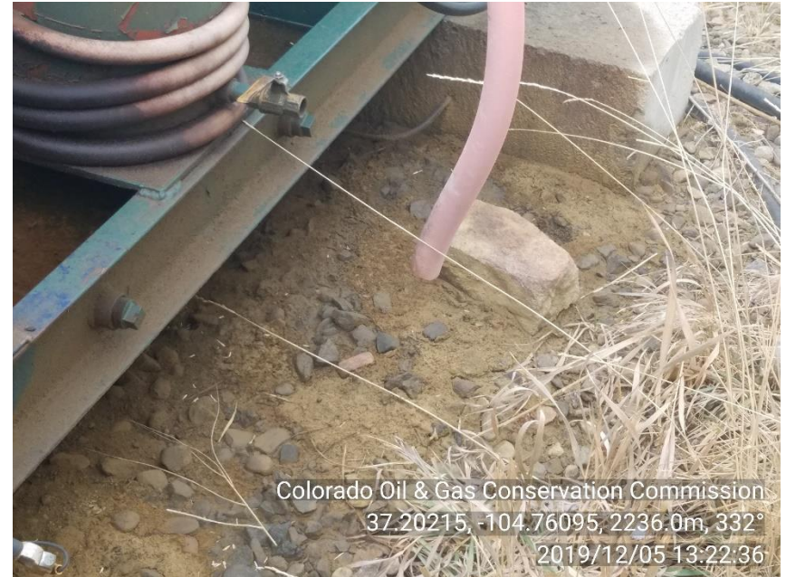
PHOTO 6: ANOTHER IMAGE OF OILY IMPACTED SOIL NEAR ENGINE SKID. Remove and dispose impacted material in approved manner, service and maintain equipment and self inspect to prevent recurrence of conditions per 1002.f(2) and 907. CA DATE 01-05-20
