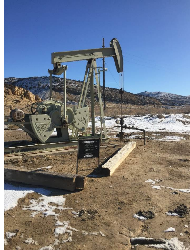
Lasso Oil & Gas location, well sign and pumping unit
