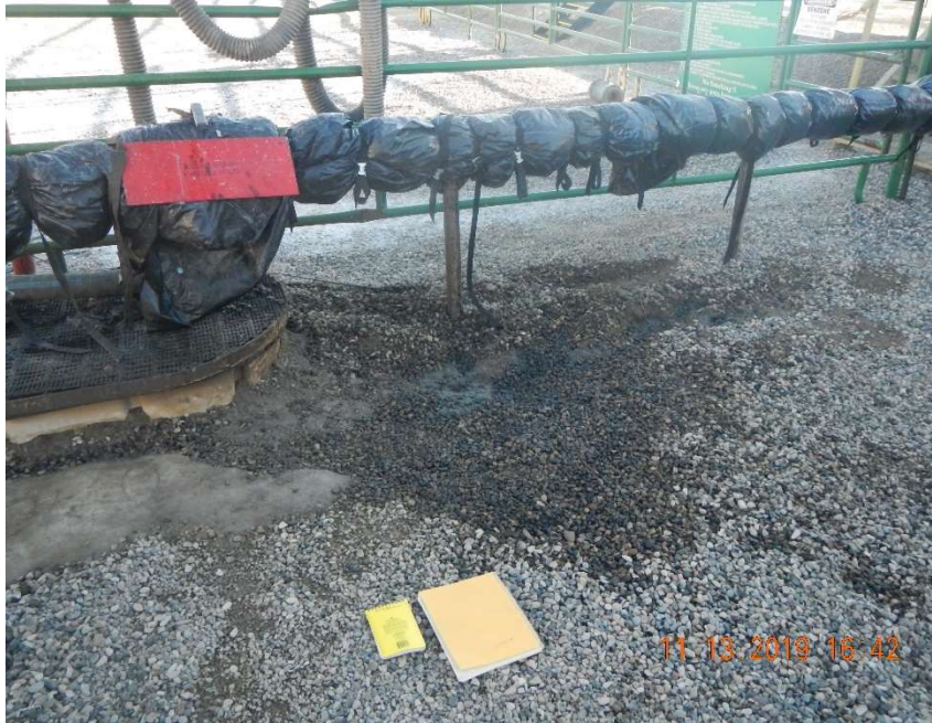
Photo #19 - View of the impacted soil around the load out area.
