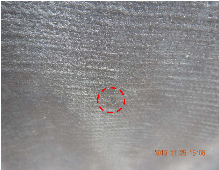
Photo #17 - Pinhole (red circle) observed in tank battery liner along south wall (2).
