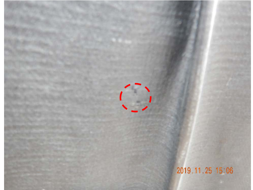
Photo #16 – Pinhole (red circle) observed in tank battery liner along south wall (1).
