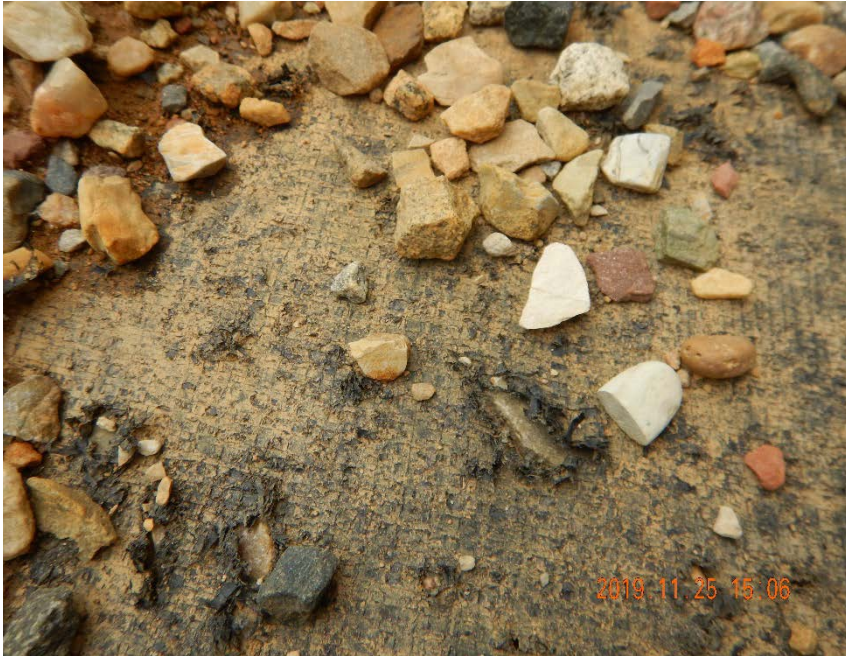
Photo #15 – Holes in base of tank battery liner beneath valve on south side of 500 bbl AST (i.e., in area circled in previous photo).
