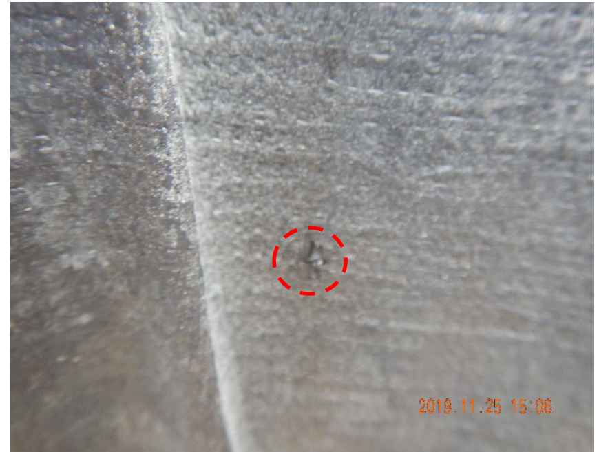
Photo #18 - Pinhole (red circle) observed in tank battery liner along south wall (3).
