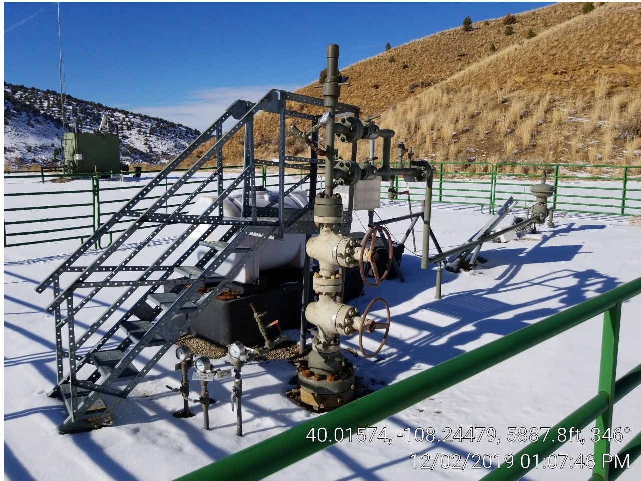
Photo 2. Well head & separator.
