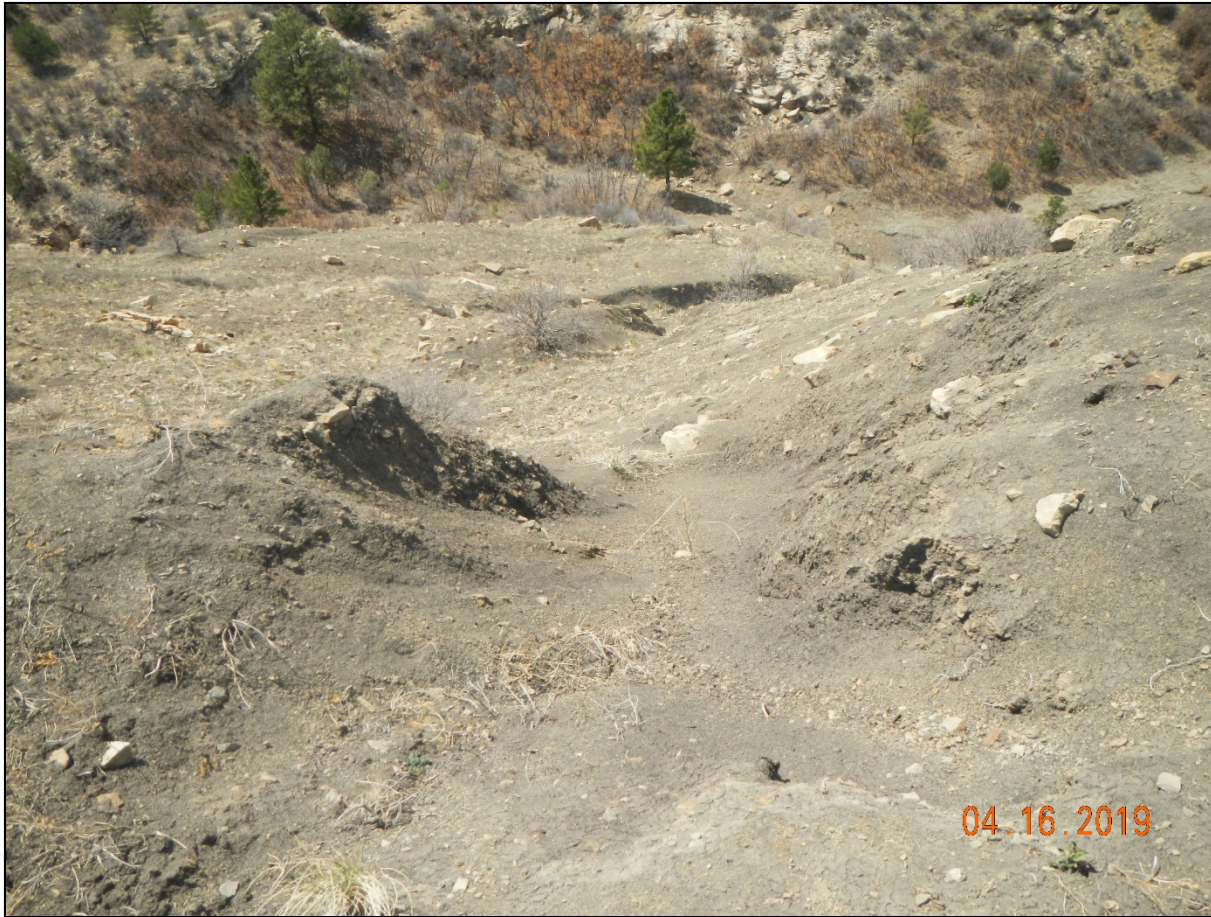
Photo 8. Facing down the fill slope shows signs of erosion.
