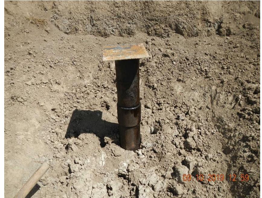
Fitzhugh #7 casing with oil staining.
