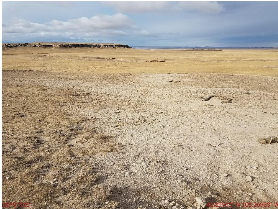
Photo 11: Photo taken from the southwest end of the pit, facing west. Photo shows wattle BMPs have not been maintained and are now debris. Photo also shows areas where reclamation has failed, and erosion degradation has been allowed to continue.
