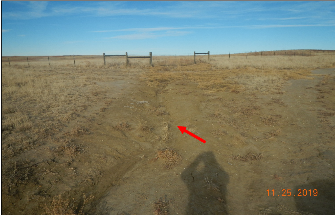
Photo 2. Facing northwest toward the location. There is erosion at the access road near the location. Vegetation has not established in this area.
