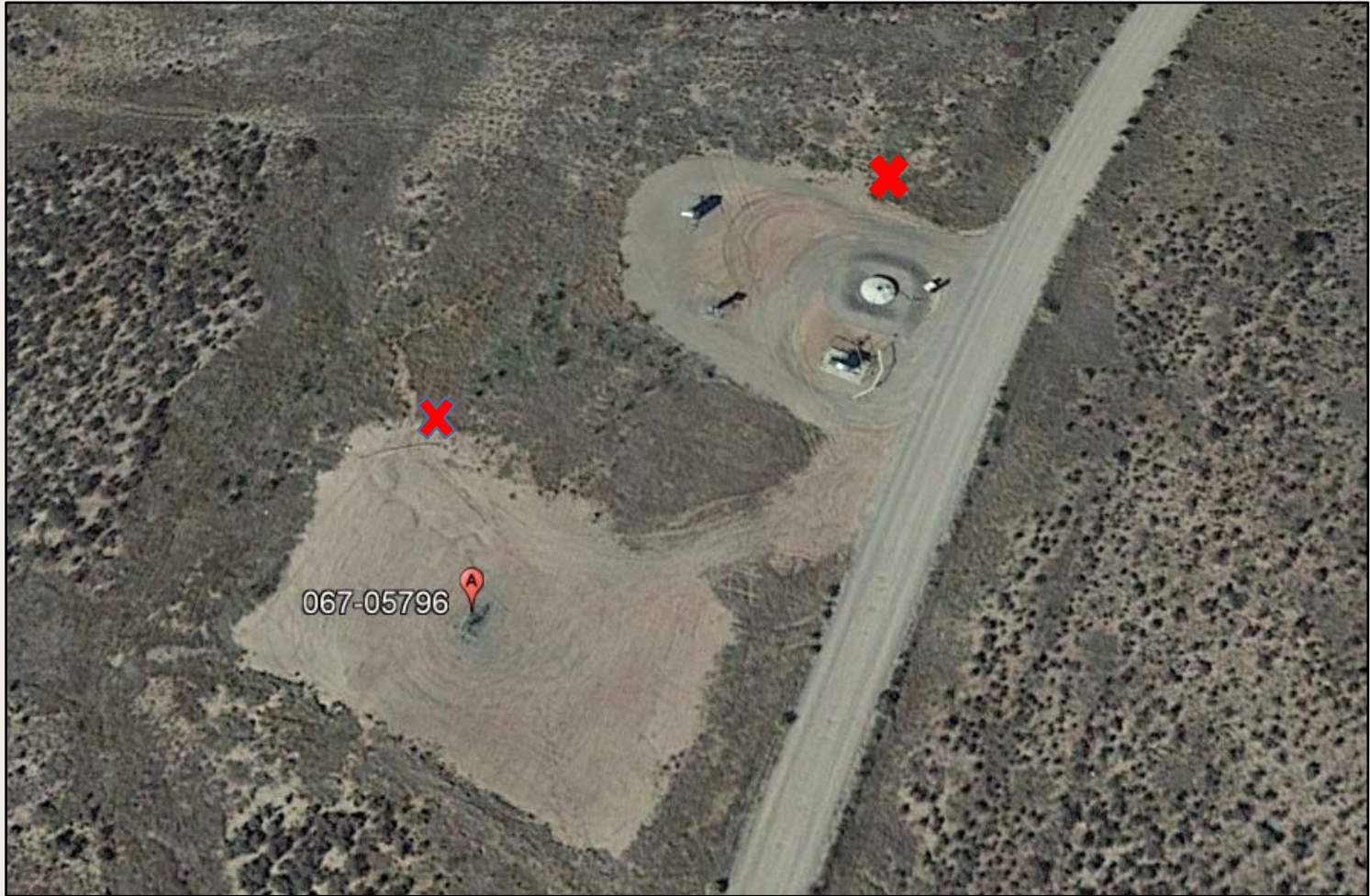
Photo 1. Aerial view of project area (2016 Google Earth). Red "X's" indicate areas within the project area where erosion and sedimentation is occurring.
