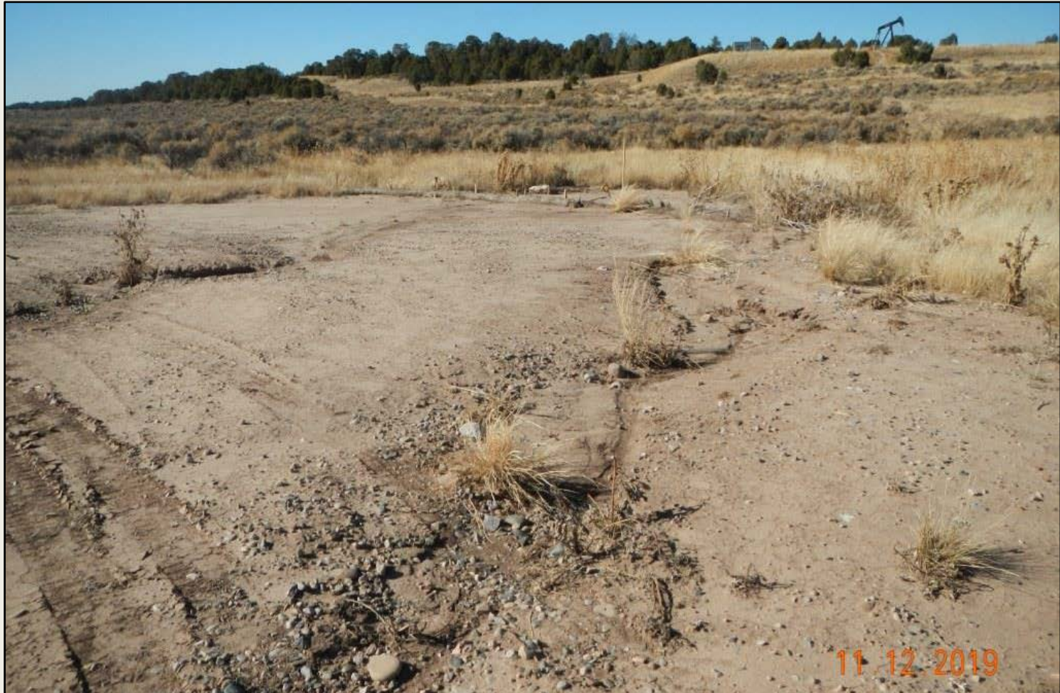
Photo 2. View of erosional channels within the western project area (northwestern corner of southern working surface). Channels are approximately 2-3 feet wide, and 6 to 10 inches deep.
