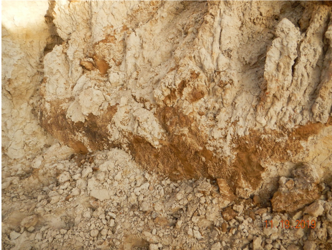
Photo # 7 – Petroleum impacted soil remains in the east wall of the pit excavation
