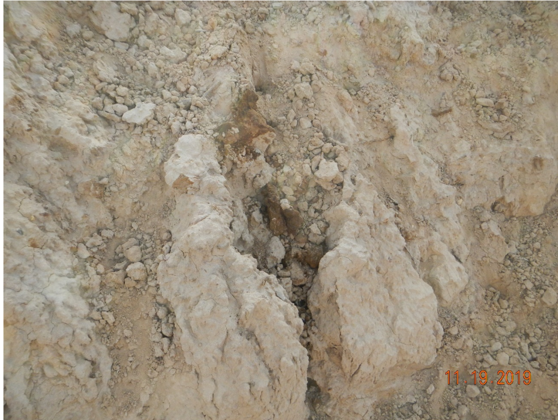
Photo # 5 – Petroleum impacted soil remains in the southwest wall of the pit excavation
