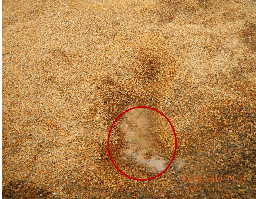
Photo #11 – View of PetroFlag sample point (Red circle) and the impacted fluids with a detectable odor and sheen located on the east side of the tank battery underneath the gravel / on top of the liner.
