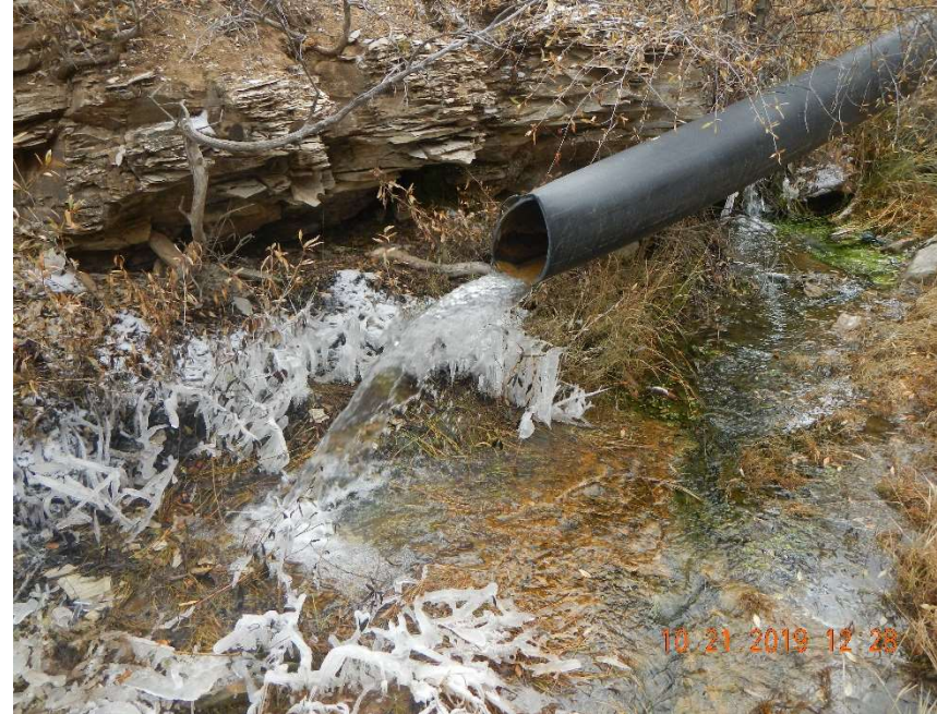
Photo #4 – View of the ruptured poly pipe.
