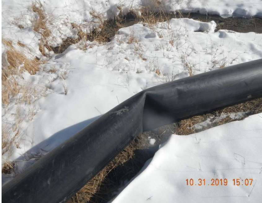
Photo #9 – View of the kink in the poly pipe.
