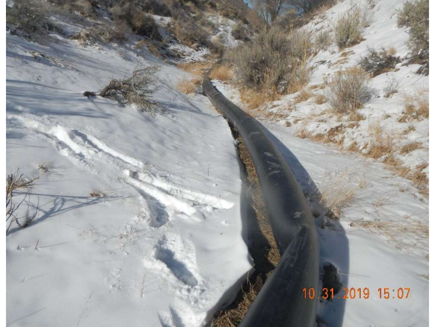
Photo #10 – View of the kink in the poly pipe looking north.
