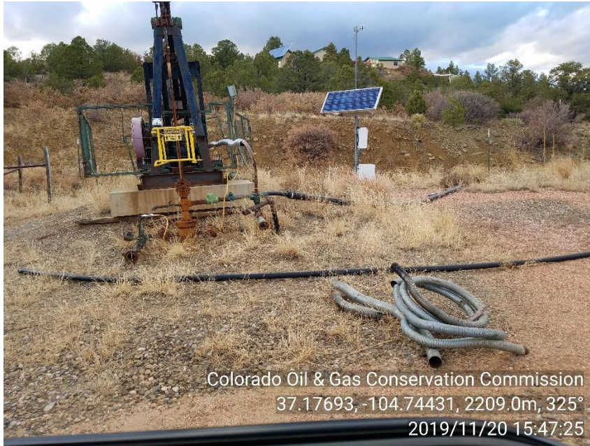
PHOTO 3: UNUSED EQUIPMENT STORED ON LOCATION (2" EXHAUST PIPE AND A 2" BLACK POLY PIPE). REMOVE UNUSED EQUIPMENT IN ACCORDANCE WITH RULE 603.f. CA DATE 12-20-19.
