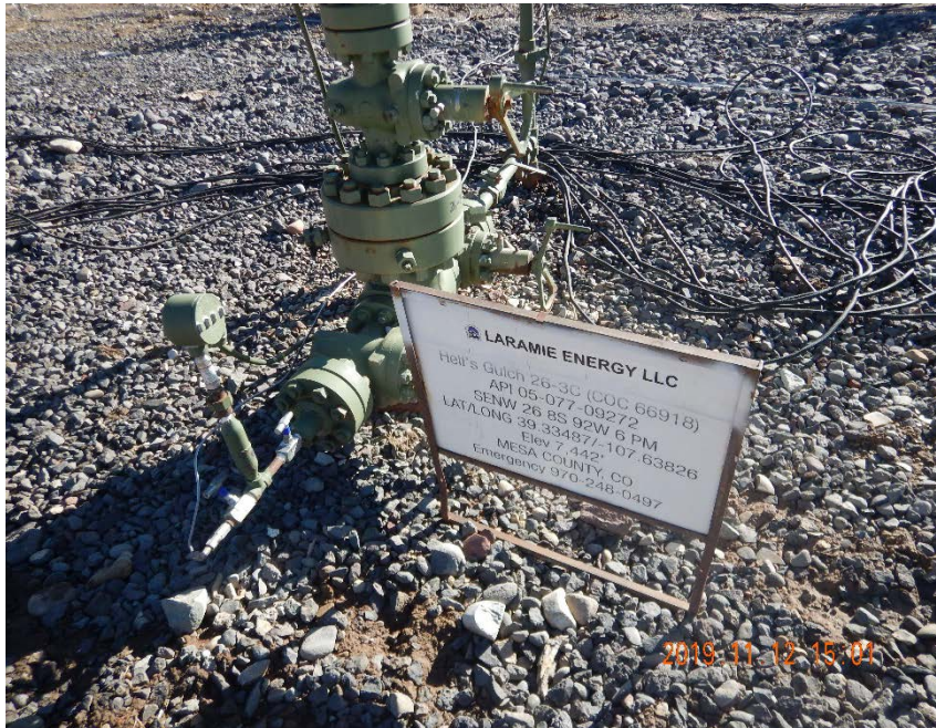
Photo #9 – Well #26-3C wellhead and sign.
