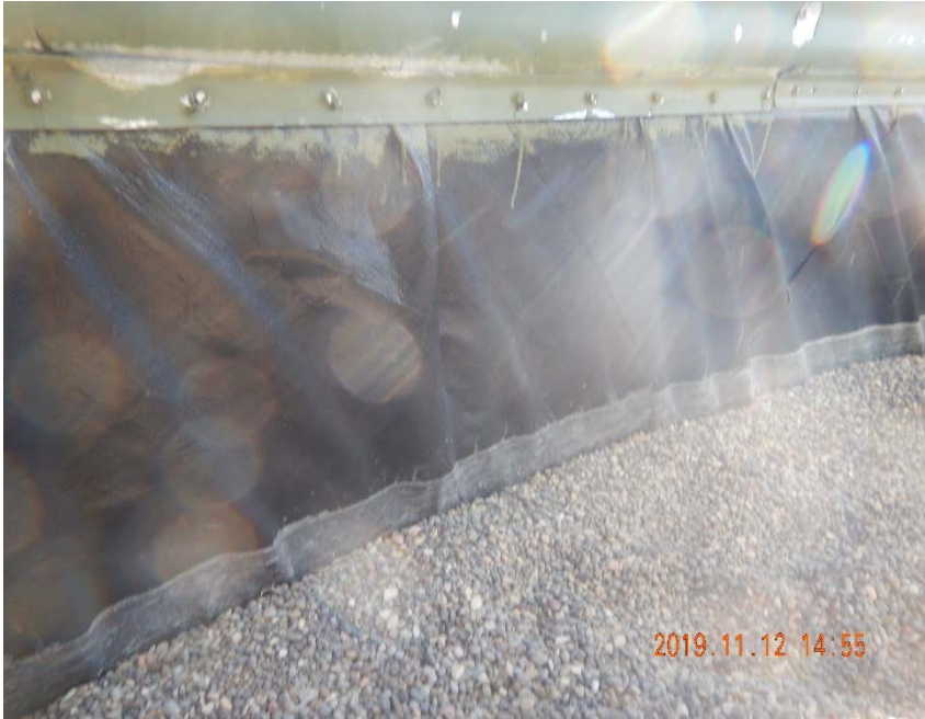
Photo #7 – Ring around base of tank battery liner indicates fluid level during release.
