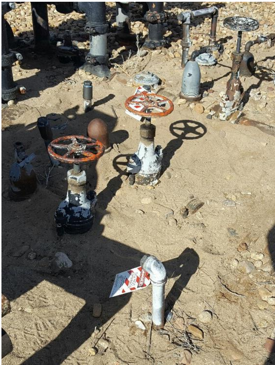
Figure #1 Risers have been bull plugged and labelled.
