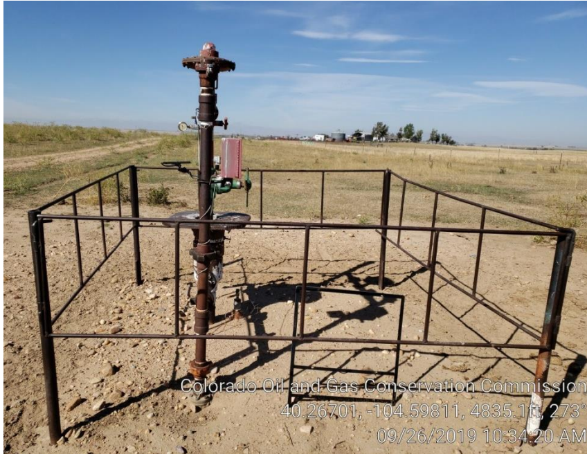
Photo #1 Wellhead & Missing sign. On 9/26/19
