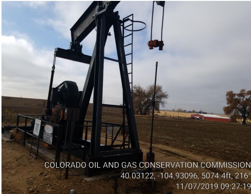
Pic 1 rods not connected to pumping unit.
