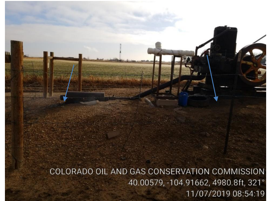
Pic 2 stained soil around exhaust and pumping unit motor
