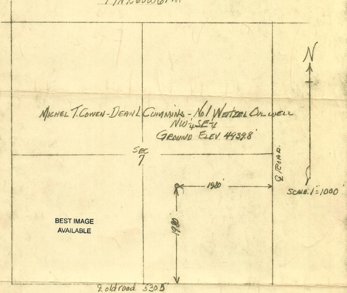
I hereby certify that the above plat is an accurate representation of a correct survey showing the location of Michal T. Cowen-Dean L. Cummins- No. 1 Weitzel Oilwell in NW 1/4 SE 7 Sec. 7 T7N R60W 6PM. The elevation of the ground at the stake is 4939.8 feet above sea level from U.S.C.&G. Bench Mark.
