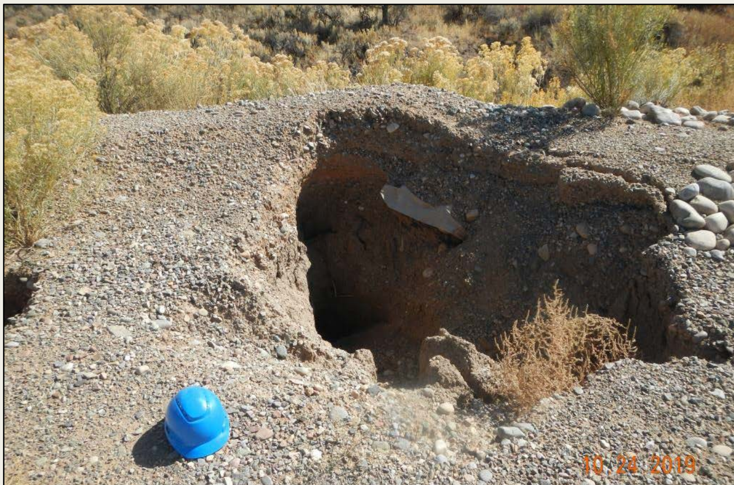
Photo 3. View of erosional tunnel approximately 3.5 feet in diameter within the eastern project area.
