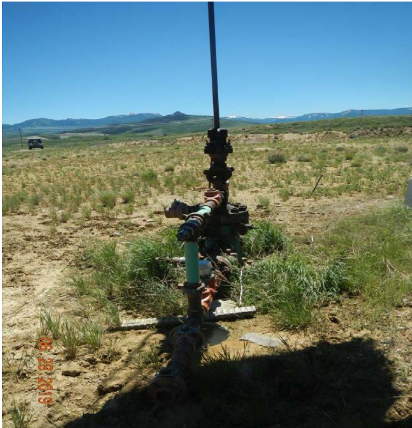
Photo#7: Rat Hole is open adjacent to Wellhead and full, with no freeboard of assumed stormwater.
